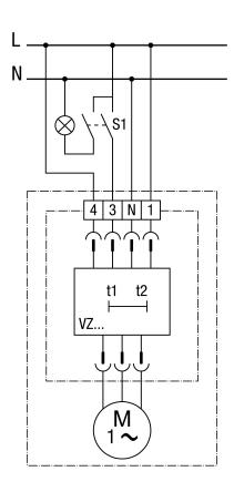
Fan always runs at base load. When the room is in use (S1=On), the fan switches automatically to full load after approx. 50 seconds.
