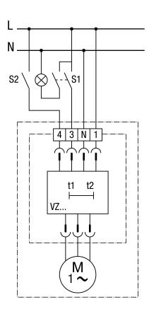
When the room is in use (S1=On), the fan switches automatically to full load after approx. 50 seconds. Base load operation can be switched off manually with switch S2.
