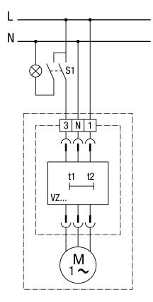
S1 on (after 0-150 s) S1 off (overrun time 1.5-24 min.) Using a 1-pin switch can cause reverse polarity voltages. Combination with an X2 capacitor necessary!
