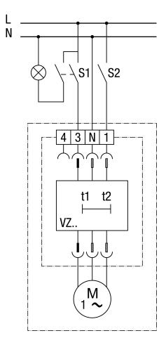
S1 and S2 on (after 0-150 s) S1 off (overrun time 1.5-24 min.) In addition, the fan can be switched off with switch S2 independent of the room lighting. Using a 1-pin switch can cause reverse polarity voltages. Combination with an X2 capacitor necessary!
