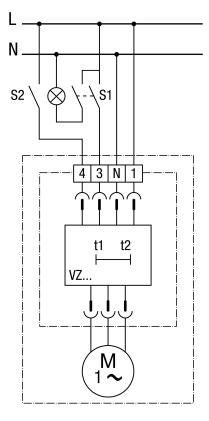
When the room is in use (S1=On), the fan switches automatically to full load after approx. 50 seconds. Base load operation can be switched off manually with switch S2. Using a 1-pin switch can cause reverse polarity voltages. Combination with an X2 capacitor necessary!
