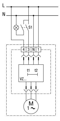
Fan always runs at base load. When the room is in use (S1=On), the fan switches automatically to full load after approx. 50 seconds. Using a 1-pin switch can cause reverse polarity voltages. Combination with an X2 capacitor necessary!
