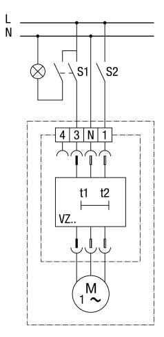
S1 and S2 on (after aprox. 50 s) S1 off (overrun time 6 min.) In addition, the fan can be switched off with switch S2 independent of the room lighting. Using a 1-pin switch can cause reverse polarity voltages. Combination with an X2 capacitor necessary!
