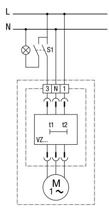
S1 on (after approx. 50 s) S1 off (overrun time 6 min.) Using a 1-pin switch can cause reverse polarity voltages. Combination with an X2 capacitor necessary!
